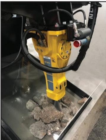
*Epiroc's SB series hydraulic breaker attachments come standard with an internal water port for dust suppression, a feature that can assist in compliance with OSHA final silica rule dust regulations.*
